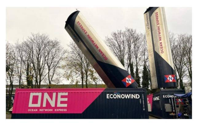
Japanese liner Ocean Network Express (ONE) is trialling wind propulsion with Dutch firm Econowind. The magenta-branded containerline is set to install two containerised wind assist devices, known as VentoFoil containers, on the *Kalamazoo*, a 1,036 teu feeder vessel operating between Busan, Yokohama, and Honolulu. The trial, scheduled to begin in January 2024 and run for approximately six months, will be a comprehensive study, with ONE closely monitoring the performance of the
