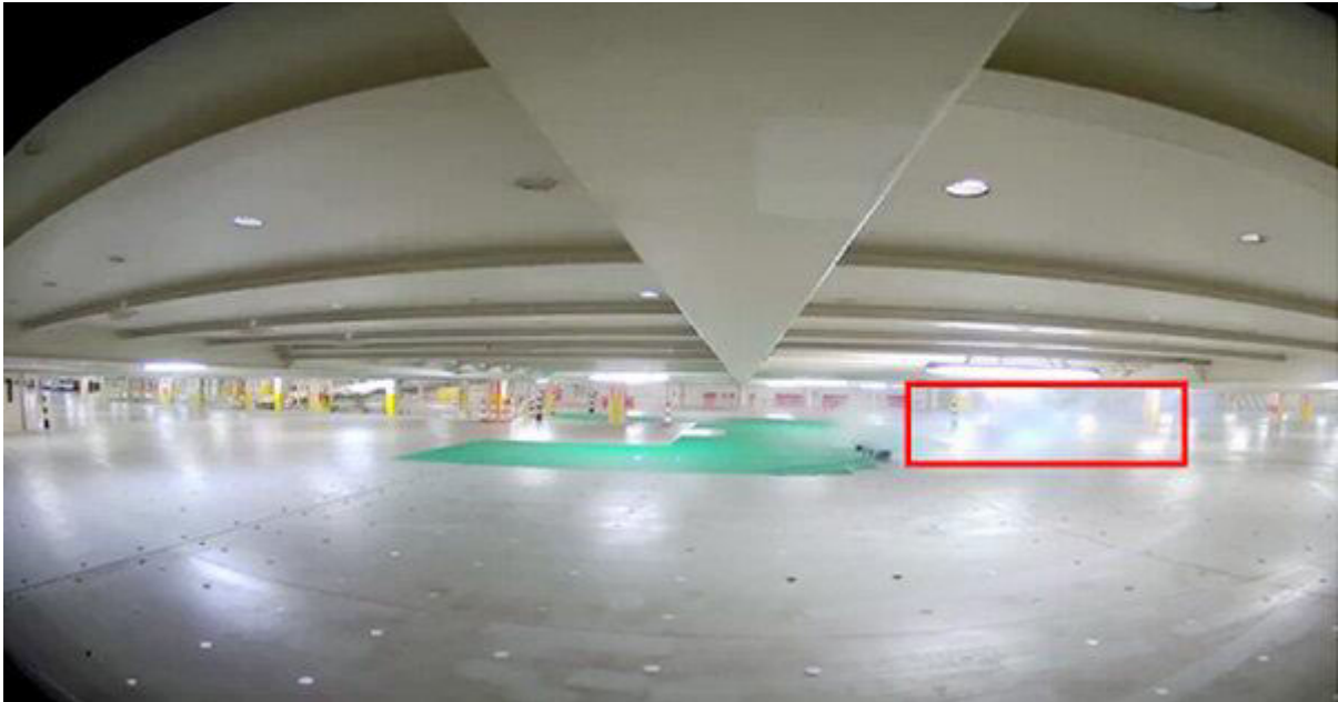
Monitor screen when detecting smoke during the test
