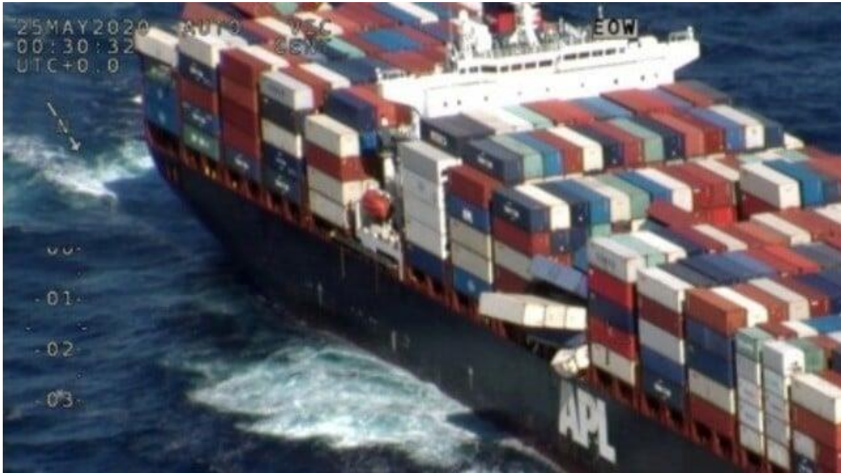
Stack collapse aboard the APL England, 2020 (USCG)
