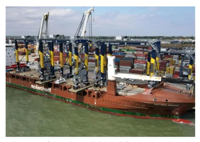
Hutchison Ports Port of Felixstowe has received its latest batch of automated electric rubber-tyred gantry cranes (AeRTGs), including five machines, which have a remote-control option.
