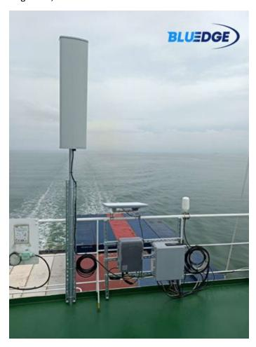
A Vessel Control Tower (VCT) hardware setup installed on a vessel's flying bridge
