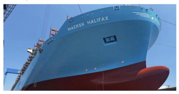
Maersk Halifax, the first large vessel in the shipping industry to be converted into a dual-fuel ship capable of operating on methanol, has completed its retrofit.
