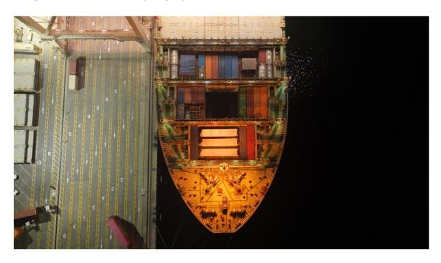
Speaking about our Special Cargo team, here's a stunning example of their work: you can see the incredible loading of 15 massive, blast-resistant modules, each weighing 23 tons and spanning over 13 meters, onto a colossal Flat Rack bed on our Haiphong Express as breakbulk cargo.
