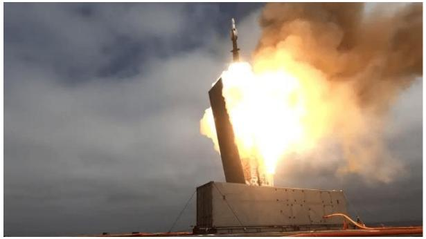
Destroyer-like armamant, small platform: a Mk 70 containerized launcher fires off an SM-6 from the helideck of LCS USS Savannah, 2023 (USN)
